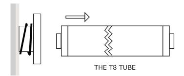
PUT ALUMINUM ROD IN THE MOUNTING HEAD
