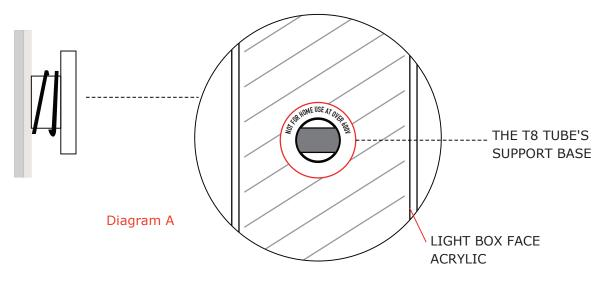
IN THIS CONDITION, YOU CAN MAKE THE TRIDENT STICK DF/SF FACE TO THE ACRYLIC BOARD CORRECTLY WITH THE HO SOCKETS.
