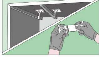
Install ArRay TOP BRACKET. Allow space around the BRACKETS. The ArRay Module Brackets are detachable, allowing for flexibility with sign box cabinet variations.
