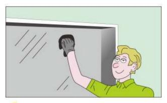
Clear sign light box cabinet of any wires, dirt or previous fixtures. Measure across to determine how many ArRay Modules across the width of the cabinet you will need
