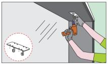
Install ArRay TOP BRACKET. Allow space around the BRACKETS. The ArRay Module Brackets are detachable, allowing for flexibility with sign box cabinet variations.
