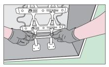
Connect the bottom bracket bar to the bottom bracket clips. Ensure the bar is fastened snugly to the module and drill the screws into the bottom bracket clips.
