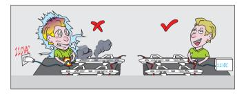
DO NOT plug in directly to a 110 VAC power supply as this will blow a fuse and damage your Modules. Damaging your modules will void the warranty. Always use the 12VDC Power Supply.
