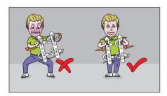
DO NOT force or twist tht ArRay Modules. To separate, simply manipulate the Modules inward to uncouple the Module Links and separate.
