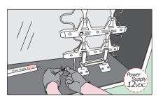
Securdly attach the wires of the final ArRay Module to the 12VDC Power Supply. Replace the cabinet cover & secure. Step back and enjoy your exceptional sign box featuring G2G Lighting ArRay Light experience!
