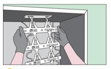
3 Affix the ArRay Module ensuring a snug fit on the brackets.
