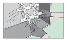
At the bottom of the sign box cabinet, affix the bottom bracket bar to the last ArRay Module.
