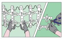
Customize the total number Modules needed. Use wire cutters to remov excess Modules and leave as much wire from the last Module (to attach later to the 12 VDC Power Supply).
