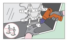
7 Affix and drill the bracket clips to the sign box cabinet to prevent the modules from shifting in the sign box cabinet.
