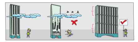
TO MAINTAIN STABILITY of the ArRay Modules in a LARGE CABINET INSTALLATION, DO NOT stack the Modules PAST 15 FEET. Add a shelf and continue with the installation.
